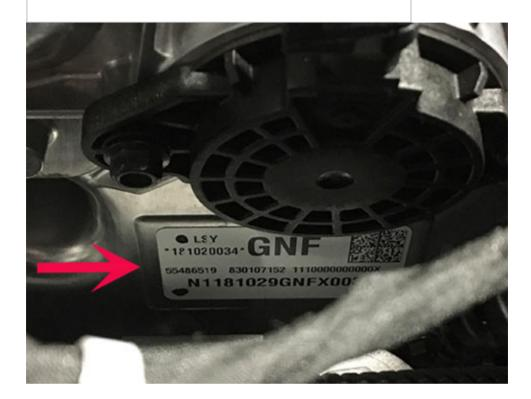
As shown in the abovephotos, the engine broadcast code can be found near the top of the engine front cover just below the engine oil fill cap.
