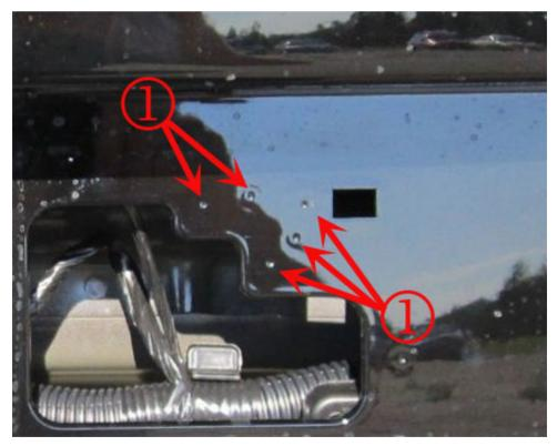
These dimples are not casting flaws in the rear fascia. They provide accurate reference for the mounting locations for various sized license plates, depending on which market the car is being driven in. Behind each of these dimples, there is a plastic boss. The plastic mounting boss behind the rear fascia can be referenced as item #2 in the following photo. Each dimple has a plastic boss behind it regardless of where it is located.
