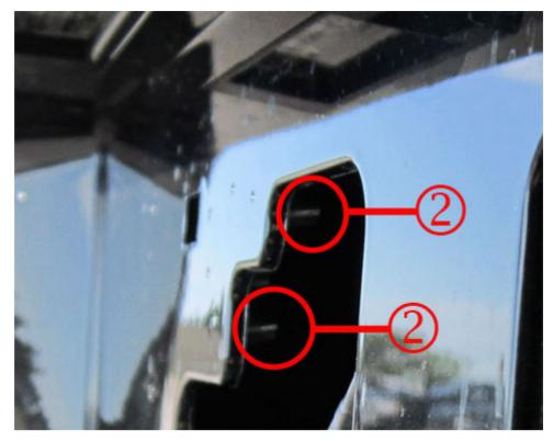
Dealership technicians are to center the license plate on the rear fascia. When it is in the correct location, technicians will confirm that a dimple is visible in each one of the license plate mounting holes. See item #3 in the picture below for an example of a correctly positioned license plate.
