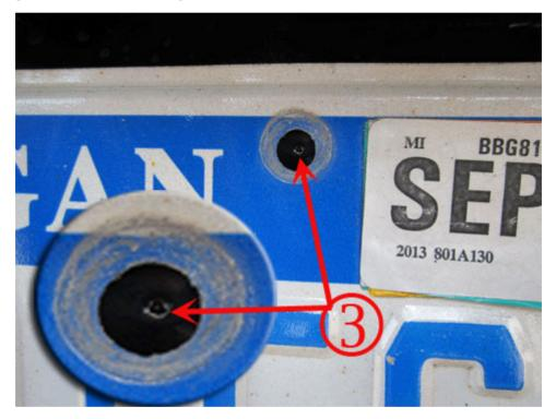
When the correct location is confirmed, take the self-tapping screws that are included in the PDI bag, and install them into the rear fascia. There is no need to pre-drill these holes. The self-tapping screws will correctly attach the license plate to the rear fascia.
