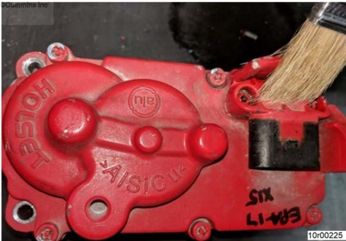
Figure 5, Cleaning VGT Actuator With Brush.
