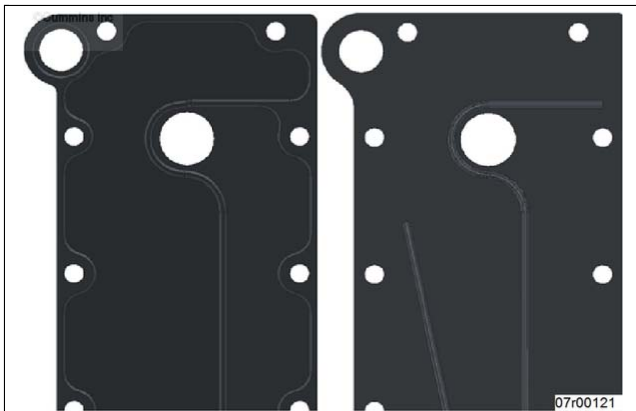
Figure 2: Left: New Lubricating Oil Cooler Cover Gasket. Right: Existing Lubricating Oil Cooler Cover Gasket.
