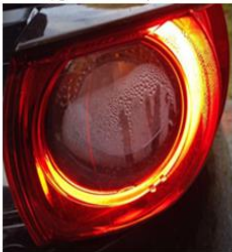
CONDENSATION RUNNING DOWN LENS - REPLACE LIGHT UNIT
