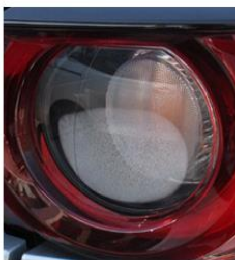
FOGGY UNIT - DO NOT REPLACE LIGHT UNIT
