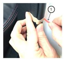
m. While holding the seaming welt so that it will not lift up, remove the red liner (1) by pulling on it.
