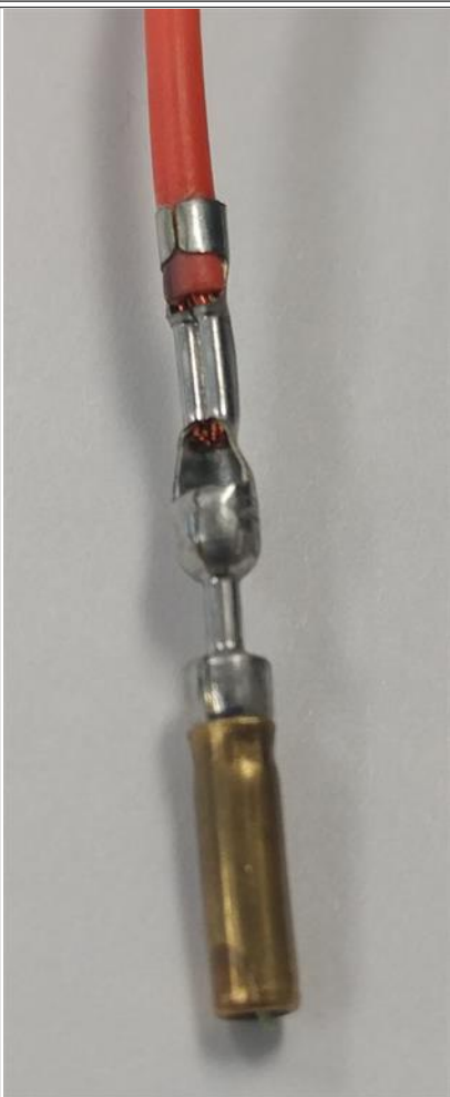
Figure 3: Terminal Properly Crimped
