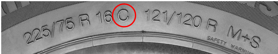
Size and Service Description of an example C-Type European Commercial Metric Tire
