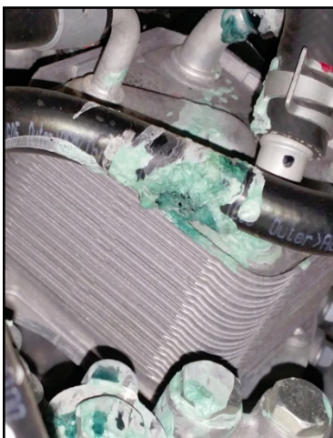
2016-2018 Outlander CVT8 Coolant Leakage
