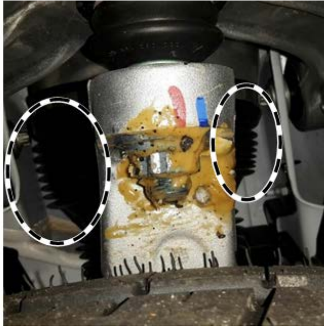
Figure 2 (Not OK, air suspension bellows significantly compressed on one side)
