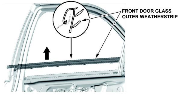
4. Lightly pull away the door weatherstrip from the top corner just enough to remove the screw on the end of the chrome molding. Lightly pull away the top end of the chrome molding, detach the clip, then remove the door sash trim.
