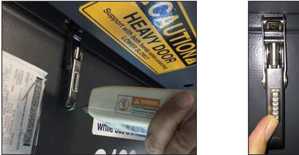
Figure 5 - Measure the Force Required to Open the Latch
