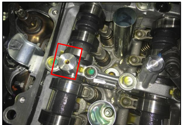
Figure 4. Cam Sensor Bolt Hole (Valve Cover Removed)
