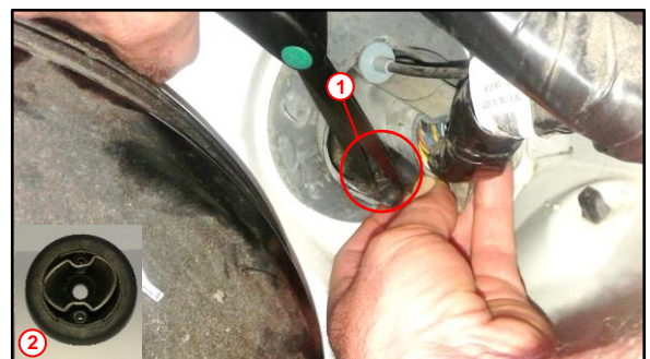
1 Cut at Grommet Indent Mark 2 Modified Grommet
