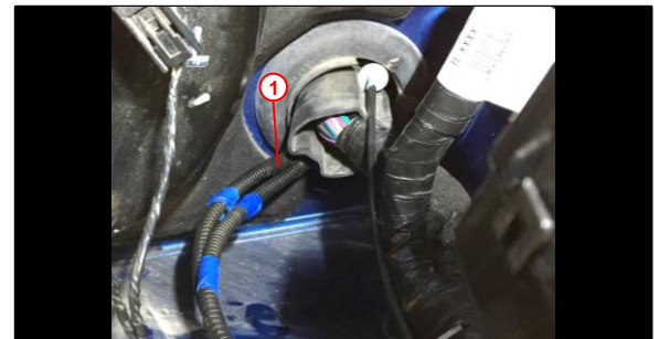
1 Engine Compartment – Corrugated Sub-Wire Harness Covers
