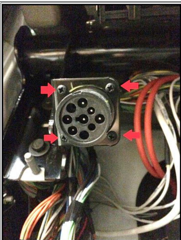
Figure #5: Secure the WYE 9 Pin
