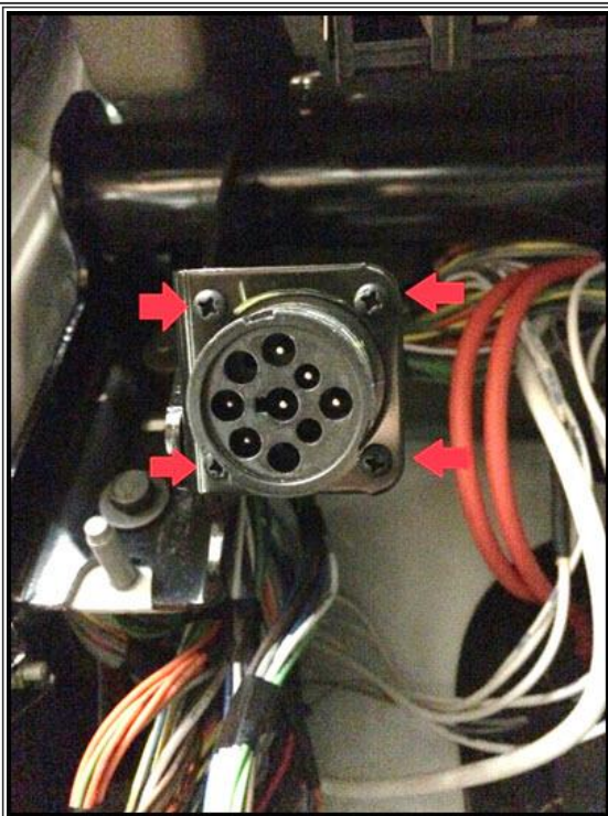
Figure #3: CAN Bus Nine Pin Connector
