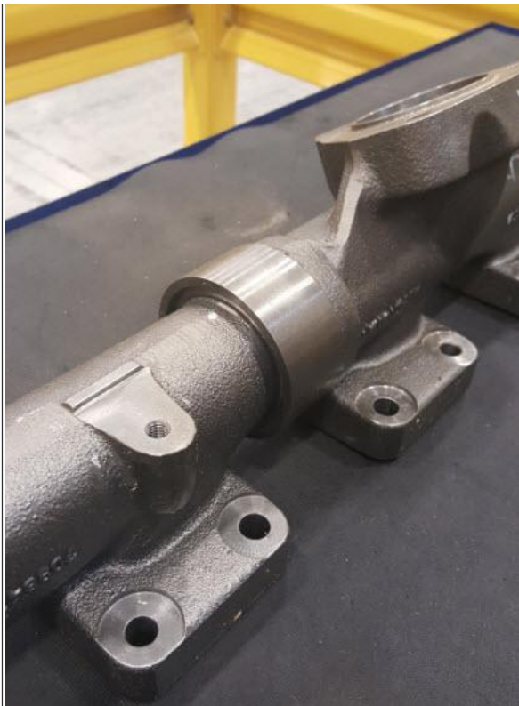
Current Manifold Joint Design
