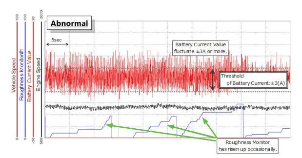
The abnormalities shown above for the Roughness Monitor and Battery Current Value are a result of resonance originating in the alternator pulley and tensioner assemblies. Although any of the listed DTCs may set, there is not an actual misfire of the engine.
