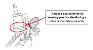
To determine if the steering gear box is a new-style unit, verify and compare the part number on the label located on the bottom cover of the pinion as shown below to the Part Information table on pg. 1. The new assemblies have been re-designed in addition to utilizing materials having improved rust and corrosion resistance.
