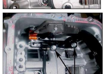
16. Connect the input and output speed sensor to the harness (see Step 13).
