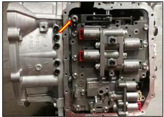
12. Remove the valve body bolts from the outermost bolts to the center bolts.
