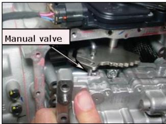
18. Install the valve body bolts and torque the bolts to specification from the center bolts to the outermost bolts.
