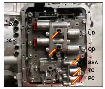
16. Refer to the DTC recorded in Step 1 and replace the related solenoid.
