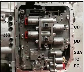
17. Confirm the O-rings are installed correctly in the case.
