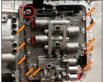
20. Reconnect the oil pressure harness to the solenoids.
