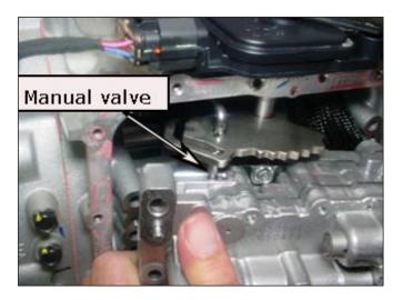
19. Install the valve body bolts and torque the bolts to specification from the center bolts to the outermost bolts.
