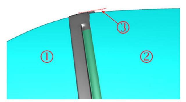
Once the quarter window is adjusted into position, compare the 2 panes of glass at the base to make sure they are flush with each other (inboard vs outboard). If the difference between the front and rear windows is more than 1.5 mm, or if there is a visible gap / daylight can be seen between the seals, the rear quarter glass needs to be adjusted further.
