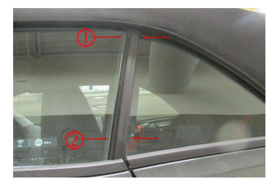
The third measurement / adjustment that must be made is the height of the rear quarter glass. It should be located so that it sits 4 mm higher than the front side window glass. This can also be seen in the following photo below.
