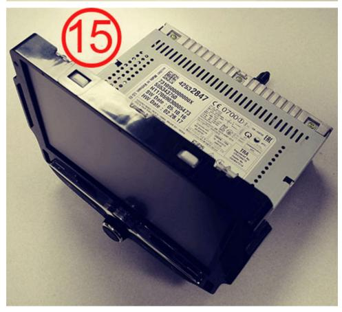
Radio Control Assembly (Corvette only)
