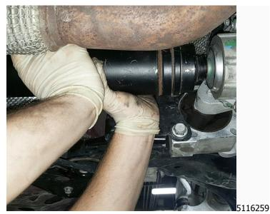
2. Using both hands, push forward firmly on the driveshaft several times as shown to ensure it is snapped into the Power Transfer Unit (PTU) fully.
