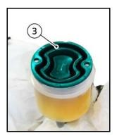
31. Locate the new *plug (A)* part no.89340291A for front brake fluid reservoir
