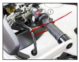
**3.** Turn handlebar straight and use a cloth to protect the parts near and under the clutch master cylinder, as shown in the figure
