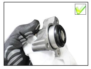
15. Install *spacer (11)* onto *clutch actuator unit (10)*, positioning it as shown in the figure
