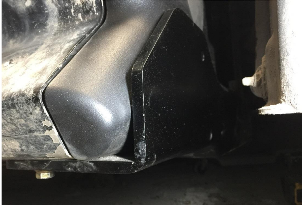
Figure 7. A closer view of the front corner guard.
