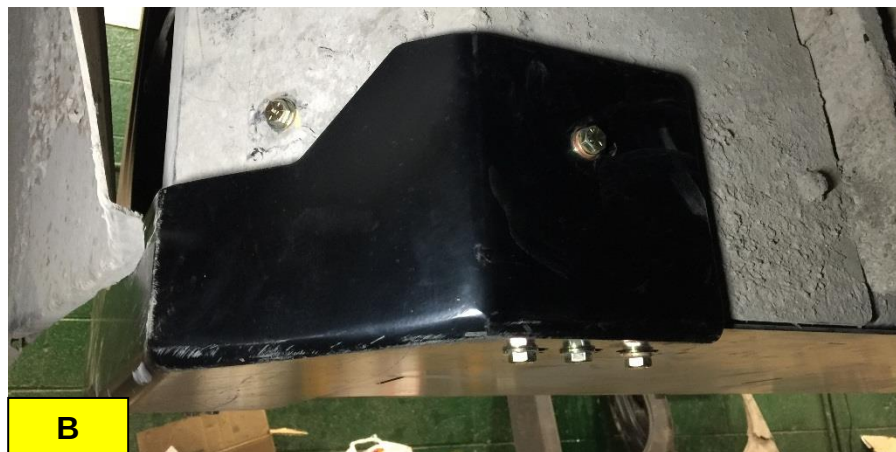
Figure 5. New shield in place near the rear of the vehicle.
