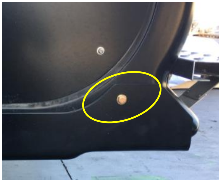
Figure 10. The corner bolt near the D-plate door is also used to attach the internal gusset.
