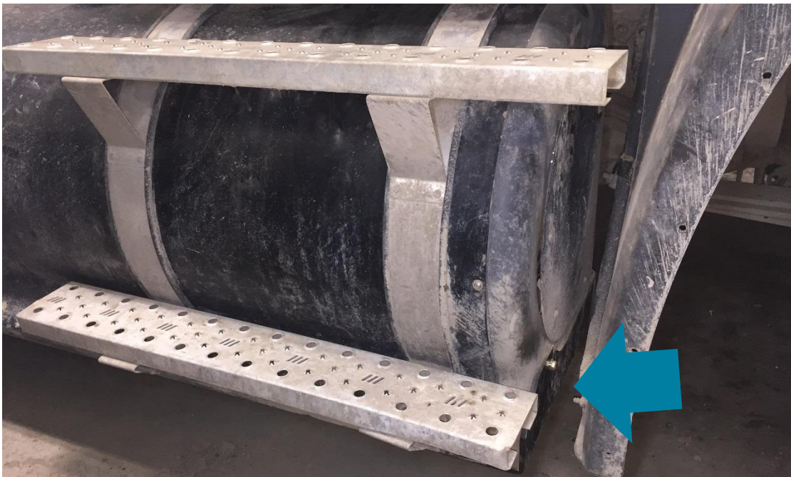
Figure 12. A view of the front corner guard. The guard is partially obscured by the step.
