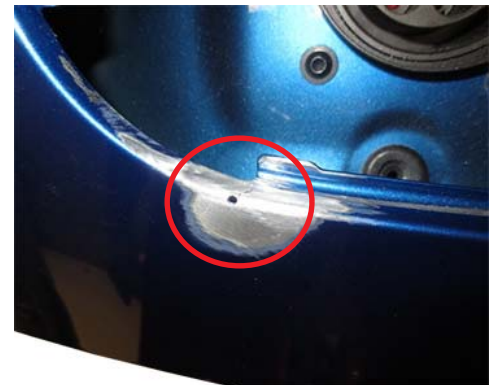
Crack sanded down and spot-drilled
