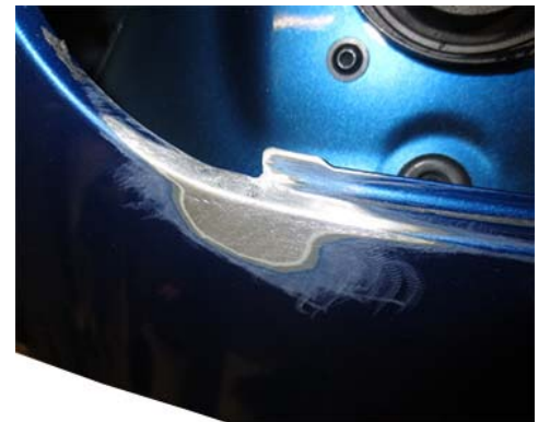
Welded seam sanded down
