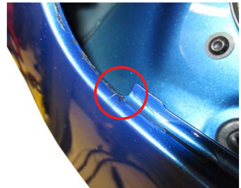
Example: Crack in rear side section
