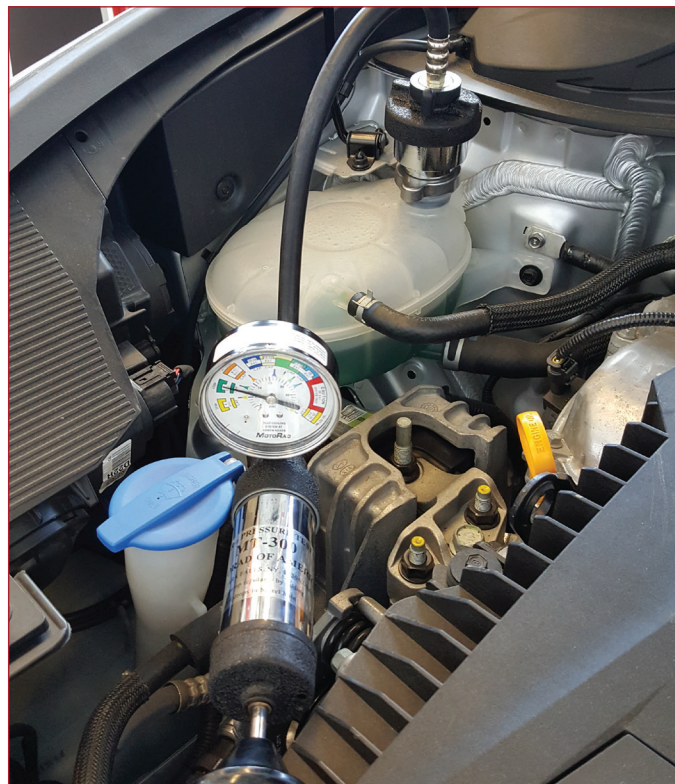
Above: Aftermarket Pressure Tester and Adapter.
