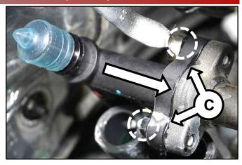
Reinstall the four (4) heater hoses in the reverse order of removal. Be sure to match and align the red and yellow markings on the lower hoses with the ATF warmer connector markings.
