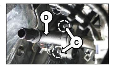
4. Be sure to remove and discard the old "brown" ATF warmer connector pipe Oring that may still be attached to the engine side of the heater pipe. The new ATF warmer connector will have a new "blue" O-ring attached to install.
