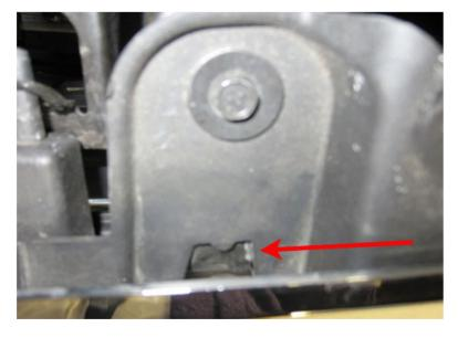
Next, with the four grille mounting bolts loose, push the center of the grille rearward and retighten the bolts. Remeasure t grille flushness. The grille should be sub-flush to the tip of the hood, as shown above.
