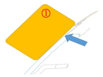
Adjust the grilleto hood relationship by first removing the sight shield. Loosen the four mounting bolts of the grille, push rearward, and retighten the bolts. Remeasure the grille flushness. If the grille is still not sub-flush as shown above, cut off the center two fore/aft locating tabs near the 10mm bolts, as shown below
