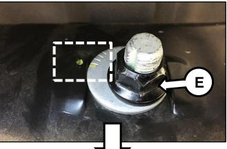
Loosen the control arm retaining nut/bolt (E) from the rear cross member.
