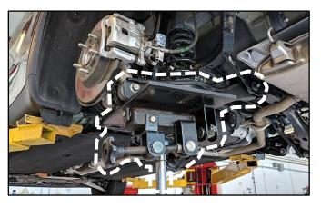
Remove the retaining lower shock bolt (A) and the stabilizer link bolt (B).
