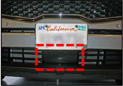
Radar module unobstructed; plate mounted correctly .
