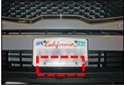
Radar module partially blocked; plate mounted incorrectly .
