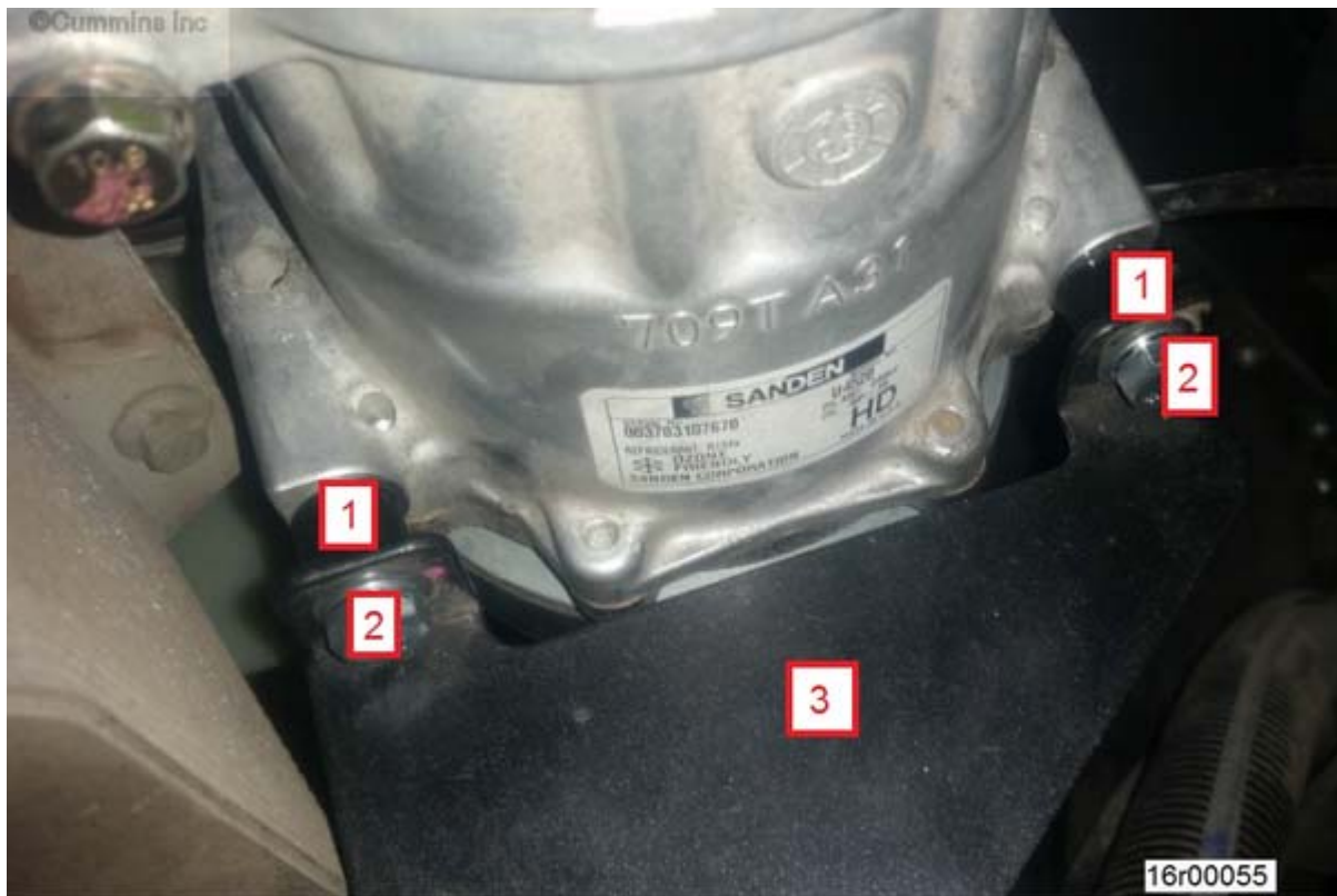
Figure 5, Freon™ Compression Lower Mount Option With Spacers Installed on Fan Shroud Support Bracket.
