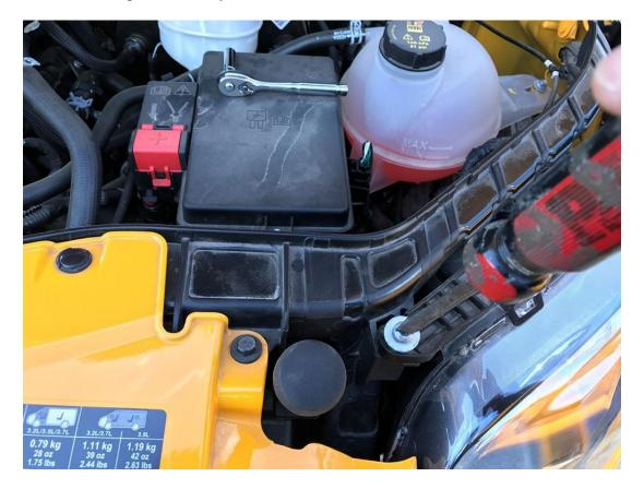
Inspecting/Securing AC Line.
