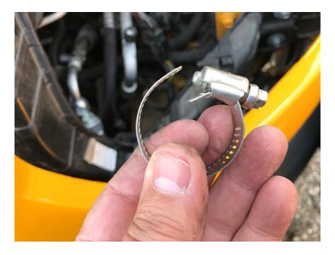
7. Place supplied clamp around protective hose and tightened at top of supplied hose. Note: Make certain there is adequate clearance between clamp and cooler.
