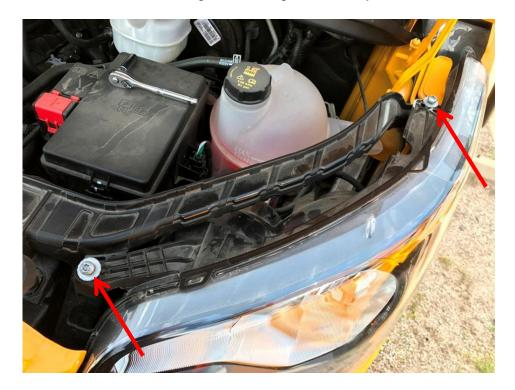
3. Remove headlight assembly to access AC line. NOTE: Pull assembly forward towards front to remove
