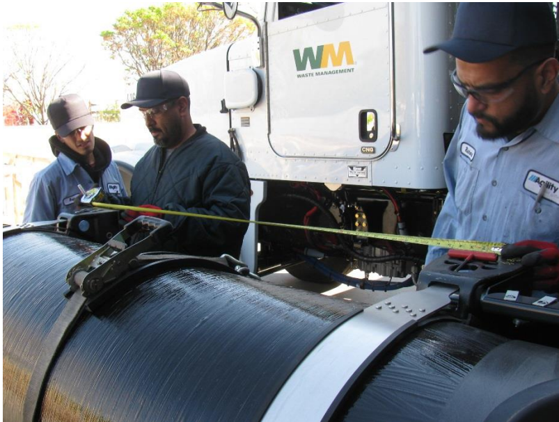
Figure 13. Measure and note the center-to-center distance between the two J-brackets. Add witness marks to indicate cylinder and strap locations to simplify proper re-assembly.
