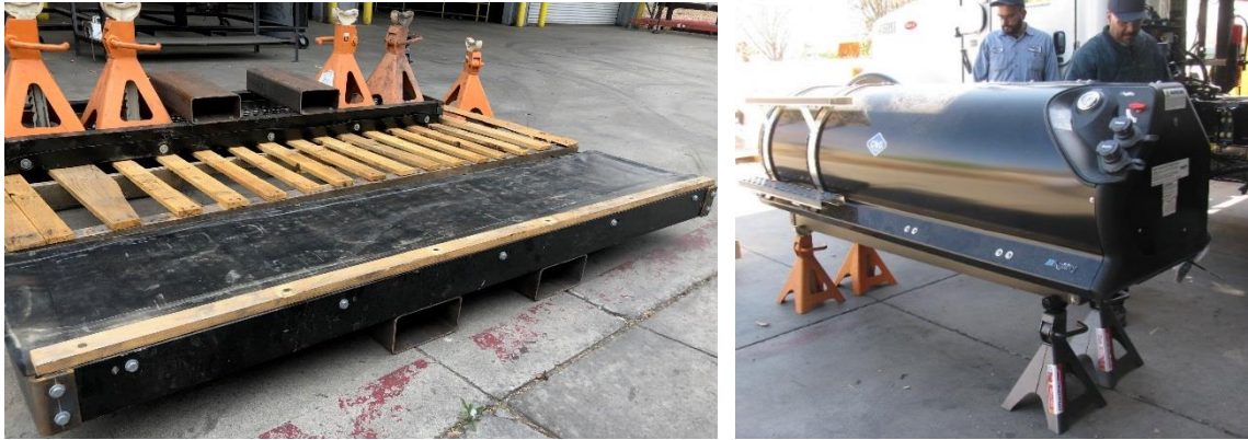
Figure 7. A cradle and lift are used to safely support the system so it can be moved away from the chassis. Jack stands are placed under the cradle to hold the system at a comfortable working height.
