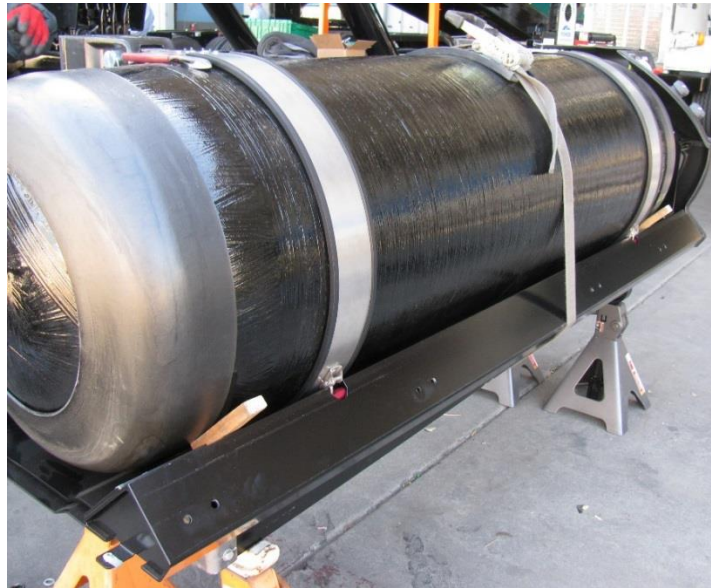
Figure 11. Secure the system on the cradle with a ratcheting strap and insert wedges along the front to hold the cylinder in place.
