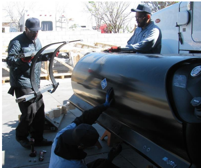
Figure 8. Time-saving tip: Remove the steps as one assembly.
