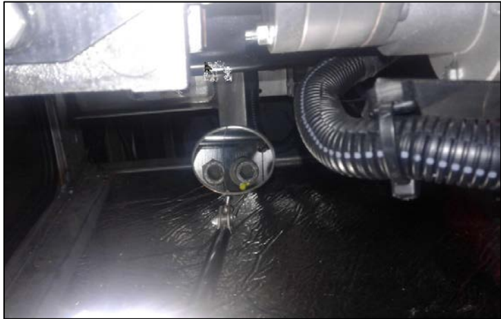
Figure 3: Using a mirror to locate the screws
