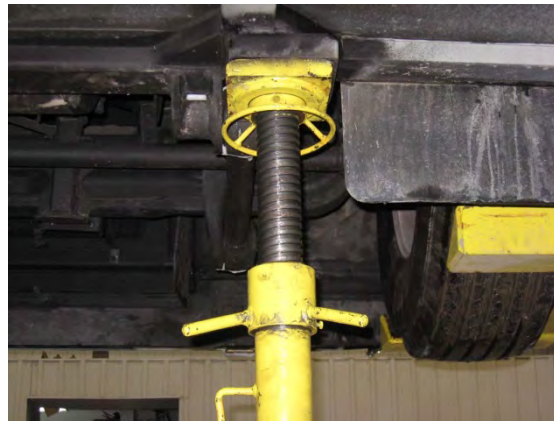
FIGURE 18 : JACK STAND AT CHASSIS HOISTING RECEPTACLE - AFT OF FRONT AXLE, CURB SIDE
