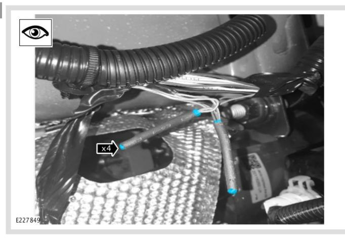
Inspect both sides of the heat shrink for 1-2 mm of glue to make sure the splice is fully sealed.
