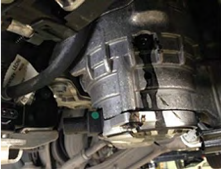
Figure 1 Active engine mount leaking oil
