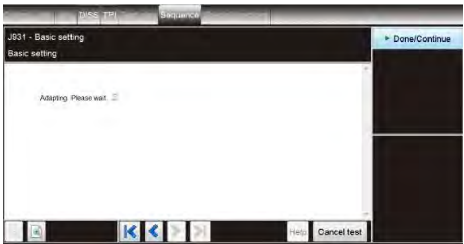
Figure 5 Follow screen prompts to complete engine mount assembly basic settings, Note: Engine mount resonance will be audible during this procedure (see Figure 5)
