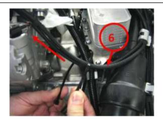
When tightening the cable tie pull the harness (6) in direction of the arrow (A/C compressor) and make sure that there is enough space between the harness and the oil cooler.
