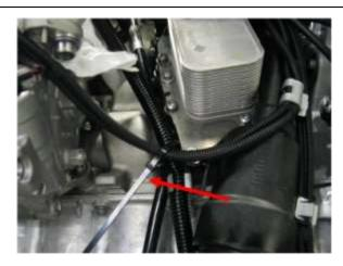
When closing the cable tie make sure that the harness does not reach into the radiator area. Cut the wire tie end off.
