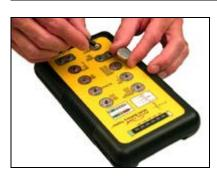
1. Place the battery (+) firmly on the appropriate test terminal.
