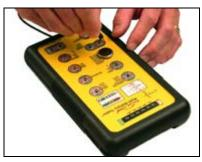
2. Hold the probe tip on the battery (-) to begin the automatic pulse load test.
