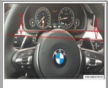
The turn signal switch and wiper switch appear uneven when the steering wheel is used as a reference point
