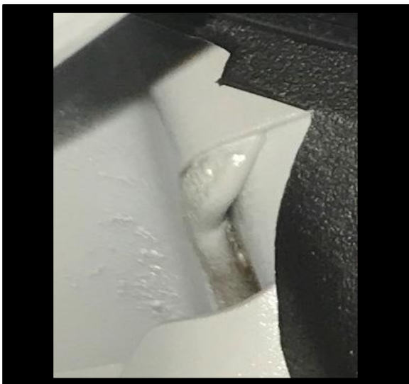
Figure 2. Body Sealer Applied Correctly on the Seam (Sealer Present Past Radius/No Gaps)
