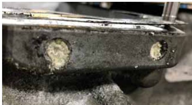
Clogged vent ports
