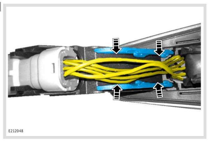
Make sure the wiring harness is positioned.
