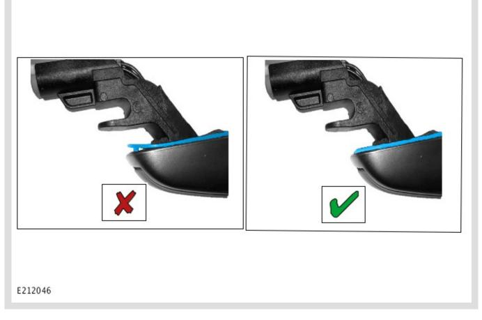
Make sure the rubber gasket sits flush against the handle base and the locating lug at the front of the gasket is installed into the hole in the handle  $(\checkmark)$ .
