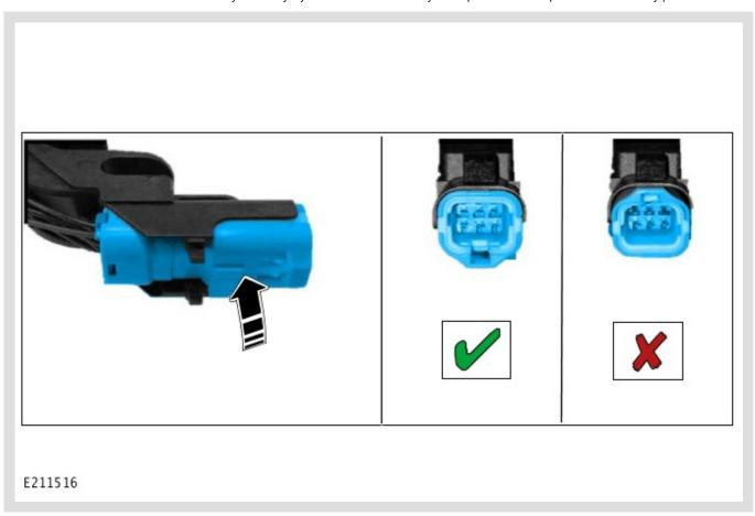
Clip the electrical connector into the handle strap inner ( $\checkmark$ ).
