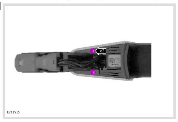
Install the 2 screws into the handle strap.
