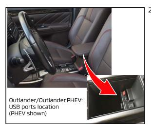
Plug in the USB flash drive containing the software update file into the vehicle's USB port (either port may be used for the update).
