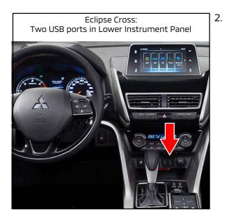
Plug in the USB flash drive containing the software update file into the vehicle's USB port (either port may be used for the update).
