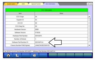
Confirm "Software Part Number" now matches the one shown for the applicable model in the "AWC ECU Reprogramming Chart" in this TSB.
