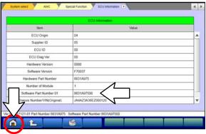
d. If the Software Part Number listed is **not** at the latest level (shown in the "AWC ECU Reprogramming Chart" in this TSB), proceed with the next step. Click the Home button to return to the System Select screen.
