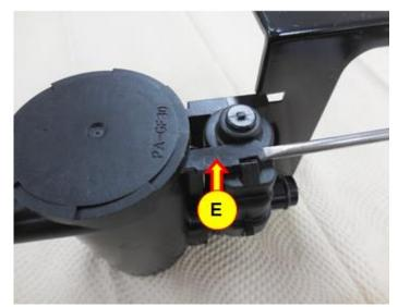
6. Rotate the CCV & bracket (F) clockwise and pull the CCV towards the red arrow direction to remove it from the fuel tank air filter (G).
