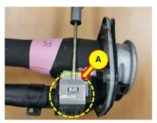
4. Pull the hose (B) in the direction of the arrow to remove the air drain case from the filler neck.
