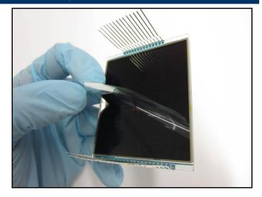
8. Carefully align the pins to the correct position.
