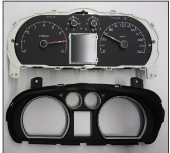
4. Use a 90 degree angle pick and carefully pry upward at the two locations (center of the LCD screen) shown in the pictures.
