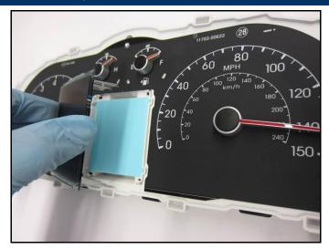
6. Lift upward and remove the blue LED light cover.
