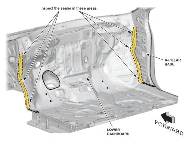
If you get a vehicle in for this, be sure to check the seam sealer in that area when you're doing water testing. If the sealer has a hole, is incomplete, or missing, thoroughly clean the area, remove any sealer that's loose or damaged, then reseal the area.
